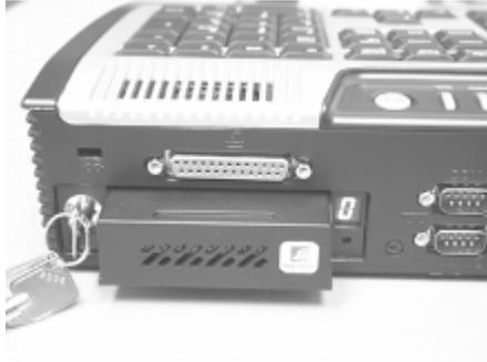
**Figure 19** Installing a Removable Hard Disk Drive
