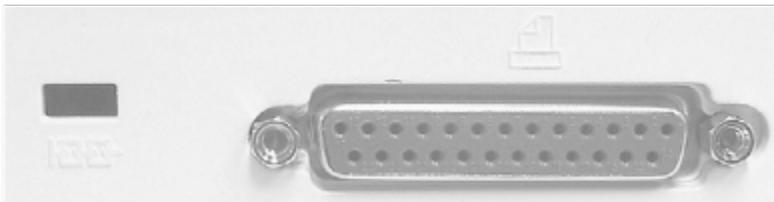
**Figure 5 Security Cable Lock Slot ♦ Parallel Printer Port**
