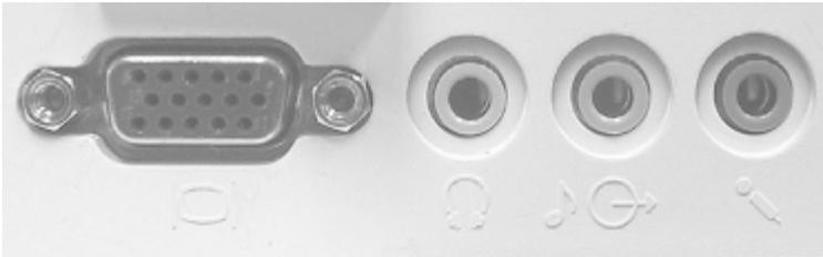
**Figure 8** VGA Port ♦ Audio device RCA jacks
