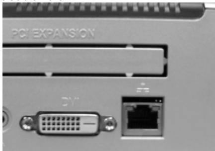
**Figure 9** DVI ♦ Gigabit Ethernet (GbE) LAN Port
